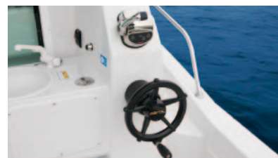
Aft deck steering station
