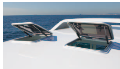
Skylight hatch (Cabin)
